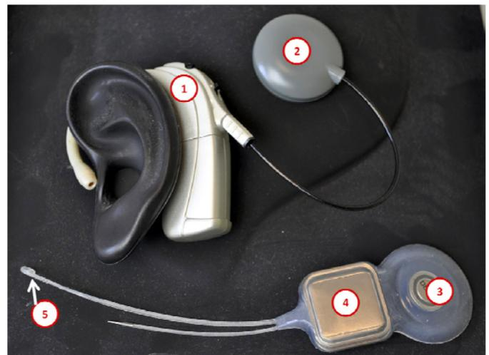
**Figure 1.** Components of a cochlear implant. (1) An external behind-the-ear processor receives sound through a microphone, processes it and (2) delivers it to the internal components through a radio frequency link. (3) An implanted coil receives the signal, and an internal device (4) converts it to electrical pulses that are delivered to electrodes in an array (5) in the cochlea.
